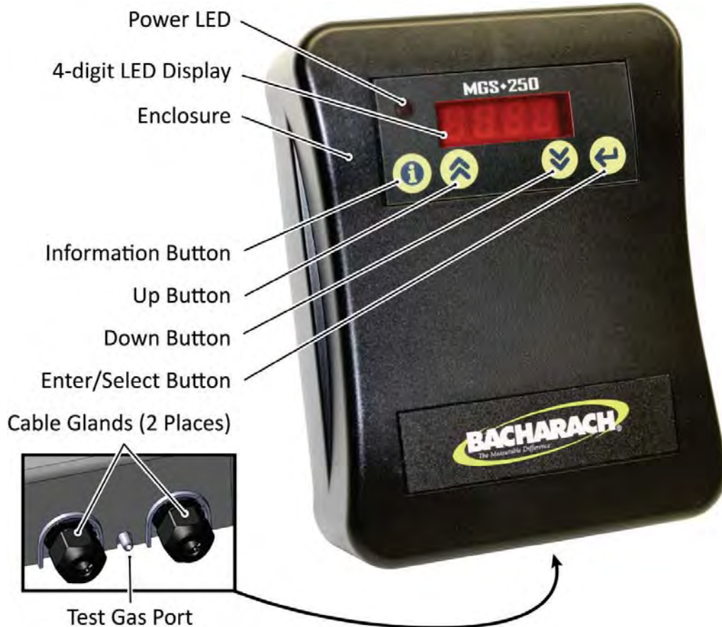
Figure 1. MGS-250 Components
