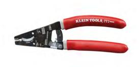
The Klein Tools Klein-Kurve Multi-Cable Cutter has a wide range of blades designed to cut multiple types of cable. The anvil cutter cuts 12 AWG copper wire and stainless steel up to 0.032-lnch in diameter. The copper curved cutter cuts 8 AWG solid and 6 AWG stranded copper wire, conductors, and coaxial cable. This tool also has a cutter for mild steel.
