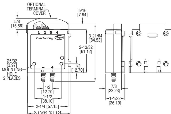
The Series 616KD One-Touch® Differential Pressure Transmitter senses the pressure of air and compatible gases and sends a standard 4 to 20 mA or optional voltage output signal. A wide range of models are available factory calibrated to specific ranges. A single push button properly adjusts both zero and span. New enclosure enables the 616KD to be mounted on a 35 mm DIN rail either via its side or back DIN rail clips.
