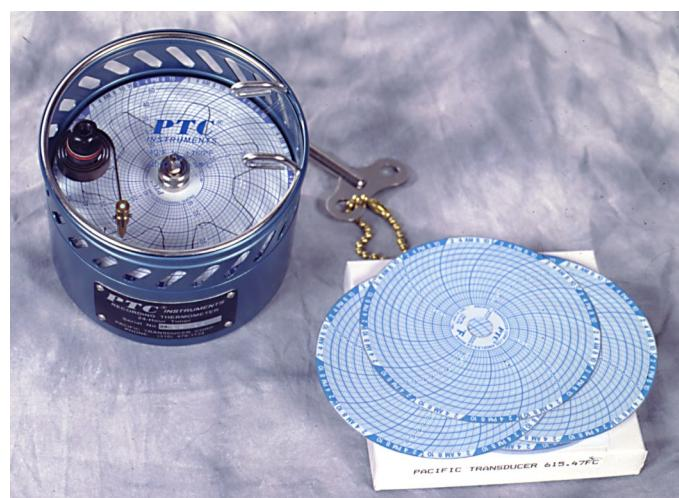
Note when used in an atmosphere where condensation might occur, the instrument must be enclosed in a polyethylene bag (see Part No. 585.86).
