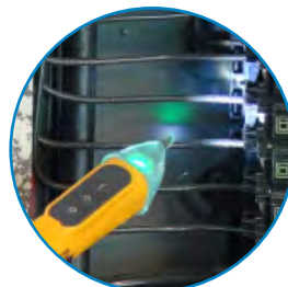
Detects AC voltage at panels
