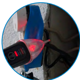
Detects AC voltage on conductors
