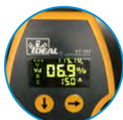
Displays Voltage Drop at 12, 15 & 20 Amps
