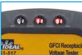
Red Lights Indicate Incorrect Wiring
