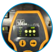
Displays H N G polarity
