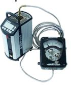
The tall CTC models with an immersion depth of 190 mm / 7.5 in are ideal for calibration of liquid filled sensors. The specially designed non-linear heating elements in the CTC-650 B and the increased block mass provide a very homogeneous temperature throughout the block. It is essential for the quality of the calibration/test that the full length of the sensing part of the sensor is exposed to the same temperature. Calibrate analog reading devices or switches with very high repeatability.
