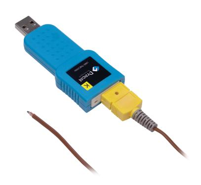
CAUTION: Keep in mind that electromagnetic interferences (EMI) may adversely reduce the precision of the sensor. Avoid using this unit close to EMI sources such as or, transformers, high voltage and fluorescent light.
