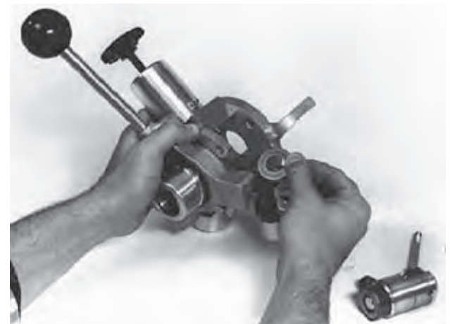
Figure 17 – Insert 2 Spacers for \frac{5}{8} " Cable
