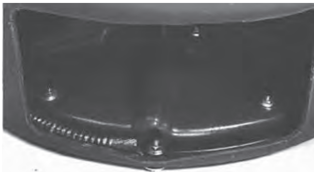
Figure 24 – Anchoring of Pigtail in Drum
