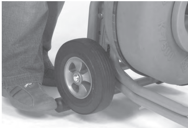
Figure 9 – Releasing Kickstand Bar
