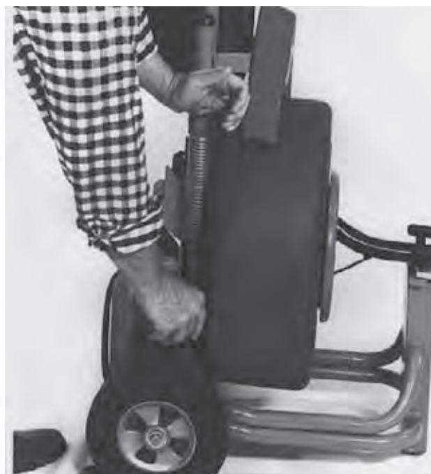
Figure 18 – Release Belt Tension
