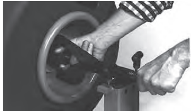
Figure 21 – Removing Knob From Center Shaft
