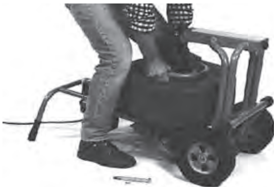
Figure 20 – Lifting Drum Assembly Onto Frame
