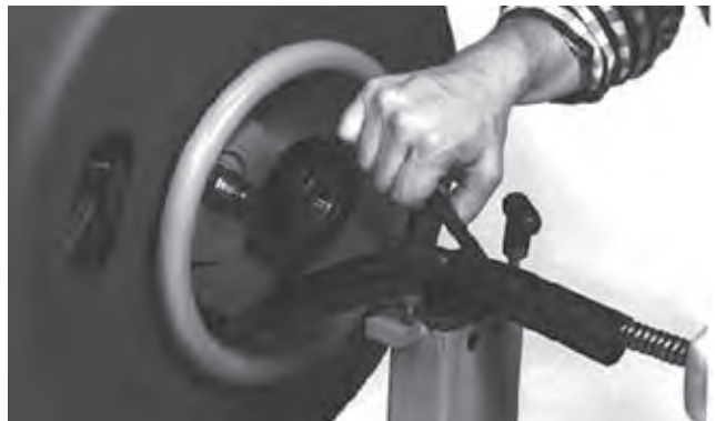
Figure 22 – Removing Guide Tube Assembly
