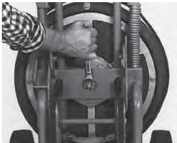
Figure 7 – Check Bolt to Ensure Tightness
