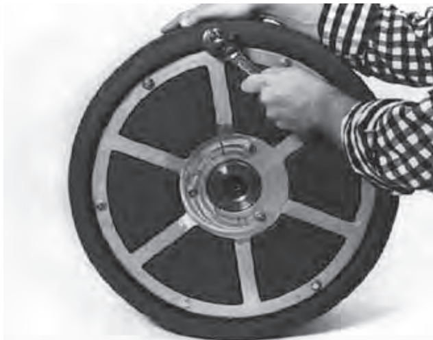
Figure 23 – Removing Pigtail Anchoring Bolt
