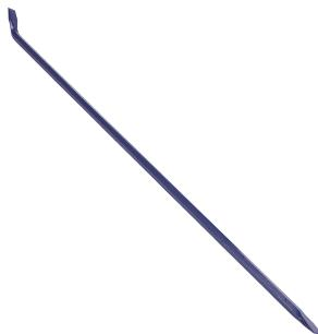
Used to lever and move objects into place with a lift and swivel motion. The hexagonal bar profile gives greater control and reduces bar roll. Forged from high-tensile carbon manganese steel for maximum strength. The heel is offset to 40° angle for optimum lifting.
