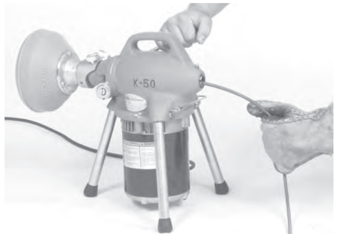
Figure 5 – Cable Adapter Attachment
