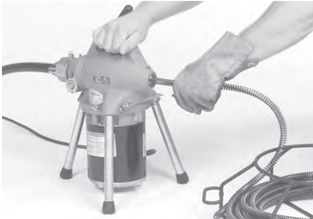
Figure 3 – Inserting Cable Into Front Of Machine
