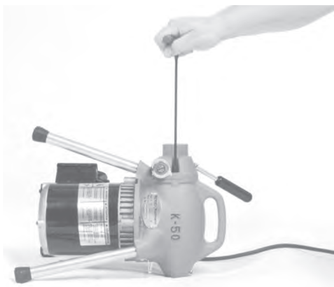
Figure 10 – Retrait des vis Allen
