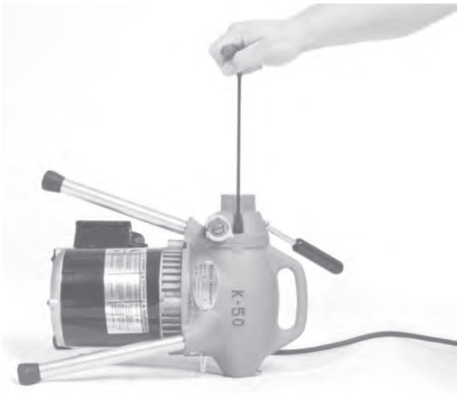
Figure 10 – Remove Socket Head Cap Screws
