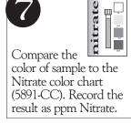
NOTE: Nitrate #2 CTA Tablets (NN-3703A) are sensitive to UV light. The Protective Sleeve (0106-FP) will protect the reaction from UV light. If testing indoors, there is no need to use the Protective Sleeve in this procedure.
