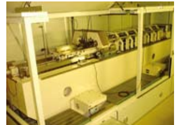
Ultra-precision length measuring machine with vacuum laser interferometer
