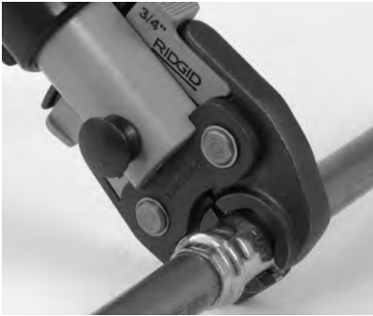
Figure 7 – Placing Scissor-Style Jaws Around Fitting
