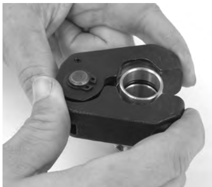
Figure 9 – Installing Press Ring onto Fitting
