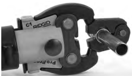
Figure 10 – Attaching Actuator to Press Ring
