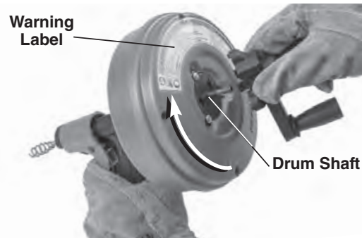
Figure 2 – Removing Crank Handle From POWER SPIN+
