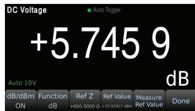
In addition to statistical data and limit test mode, this series is capable of Null, dB, dBm, mX+b, run/stop, and percent calculation functions.
