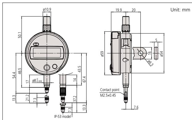
Note 1: Dimensions of the inch (ANSI/AGD Type) dial indicator partly differ from those of the metric (ISO/JIS Type) indicator.
