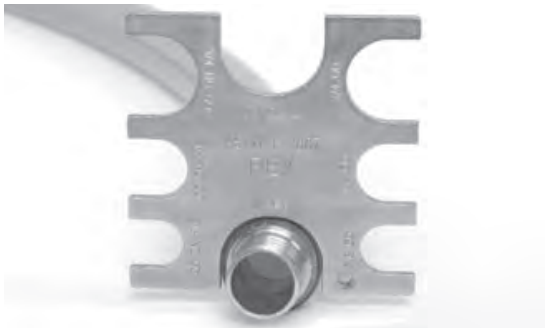
Figure 11 – Correct Go Gauge Fit
