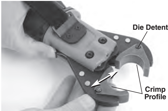
Figure 7 – Removing and Installing Dies
