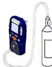
Figure 4.1 Bump Test / Gas calibration set up
