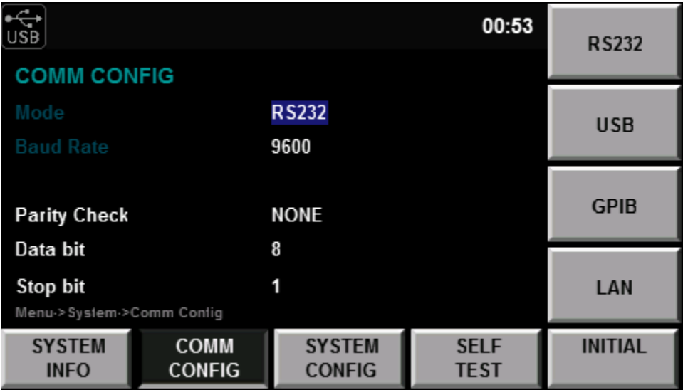
Figure 2.3 COMM Configuration - RS-232
