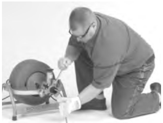
Figure 7 – Proper Operating Position
