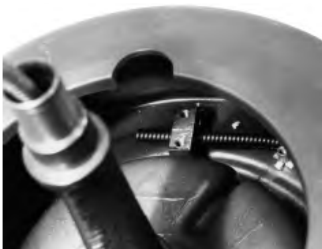
Figure 16 – Position New Cable Under Bracket
