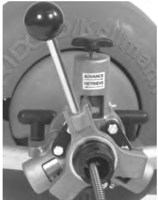
Figure 9 – Autofeed in Reverse Position
