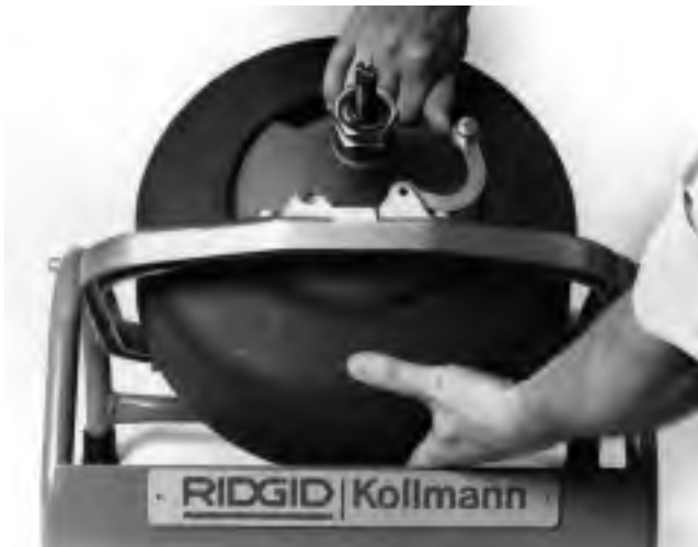
Figure 2 – Aligning Drum and Gearbox Bore
