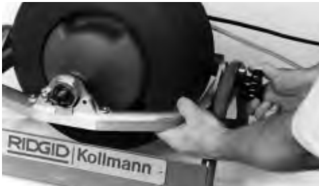
Figure 1 – Pivoting Yoke Assembly
