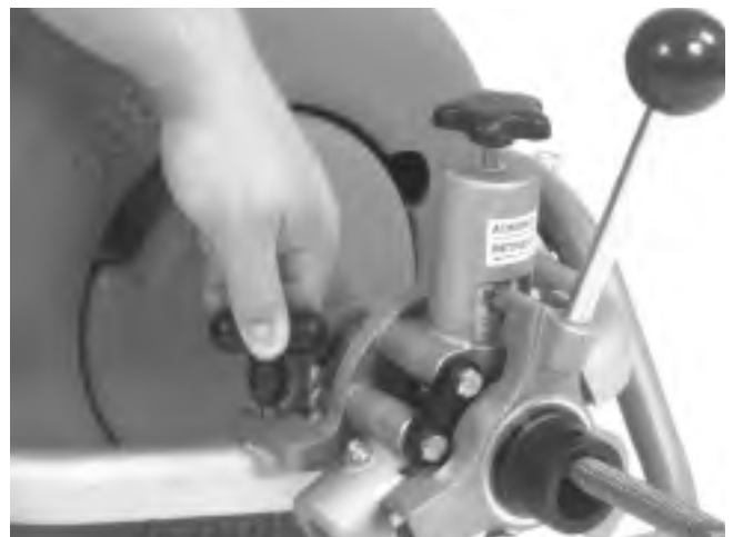
Figure 4 – Mounting the Autofeed Onto the Frame
