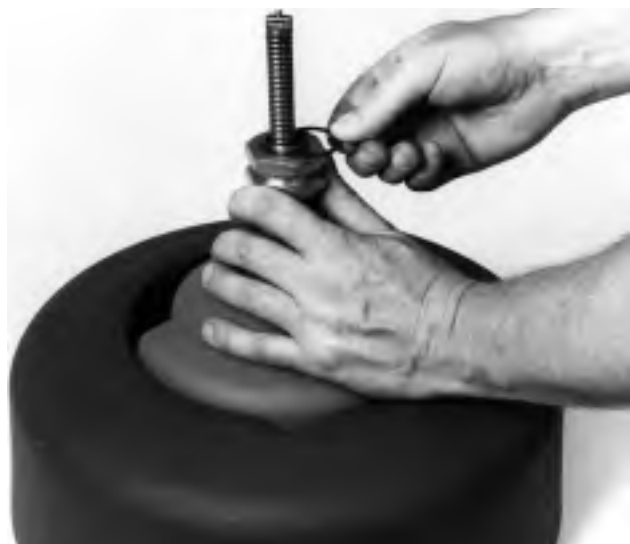
Figure 17 – Reassemble Inner Drum, Front Bracket and E-Clips
