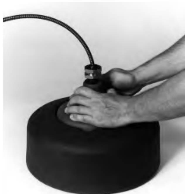
Figure 13 – Removing Cable End
