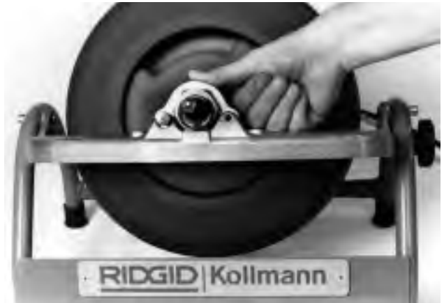
Figure 3 – Locking Front Bracket
