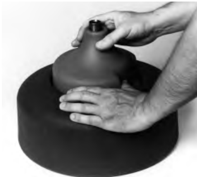
Figure 15 – Removing Inner Drum
