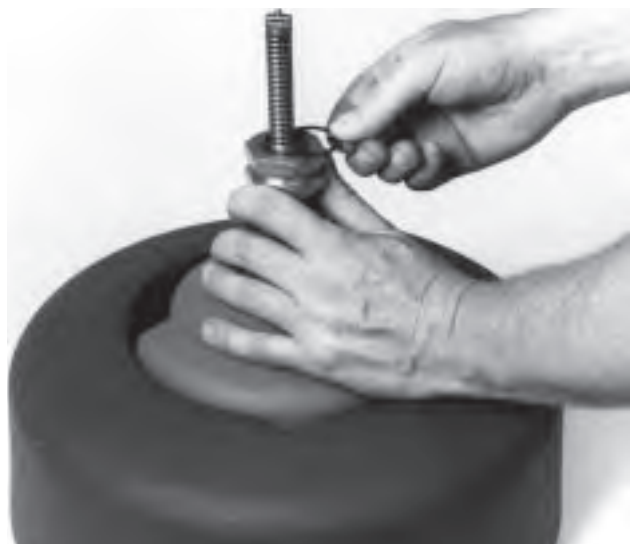
Figure 17 – Reassemble Inner Drum, Front Bracket and E-Clips
