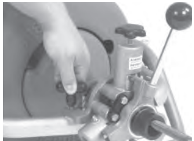
Figure 4 – Mounting the Autofeed Onto the Frame
