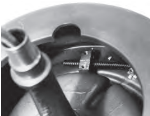
Figure 16 – Position New Cable Under Bracket
