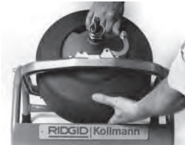
Figure 2 – Aligning Drum and Gearbox Bore
