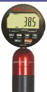
ASTM Type D Durometers are for determining indentation hardness of Pipeline Coating, Hard Rubber, Acrylic, Delrin, Kevlar, PVC, Nylon, Lexan OUAL THE WAY AGENEN and Epoxies.
