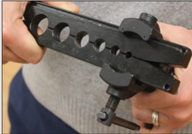
Railing allows yoke to smoothly travel while keeping the flaring tool and bar aligned
