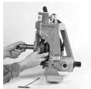
Figure 18 – Removing Retaining Shaft and Groove Roll
