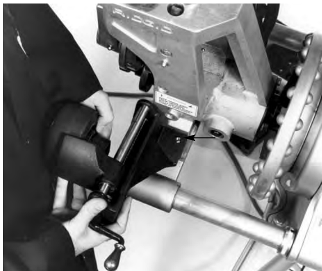
Figure 22 – Line Up Bolt Holes in the Mounting Bracket with Bolt Holes in the Base
