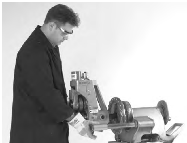
Figure 2 – Installing on 300 Power Drive
