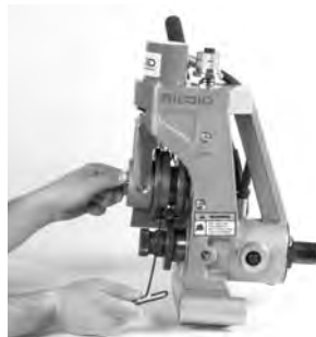
Figure 17 – Loosening Grooving Roll Set Screw
