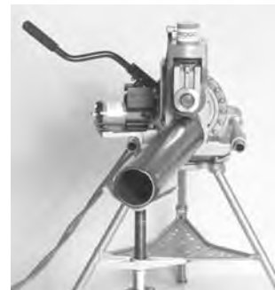
Figure 13 – Offset Pipe on 918 in REVERSE Position
