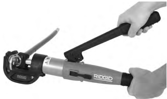
Figure 7 – Using Crimp Tool
