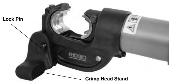
Figure 5 – Installing the Crimp Head on the Stand
