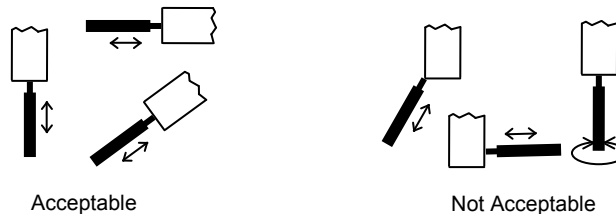
Figure 1 – Correct and Incorrect Angles of Measurement
