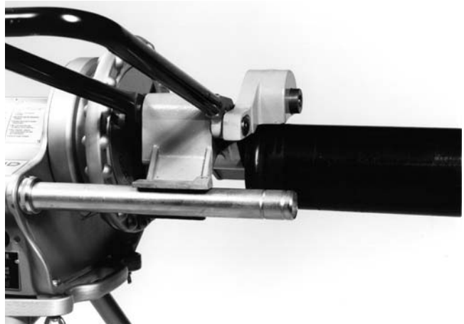
Figure 6 – Square Pipe & Pipe Support
