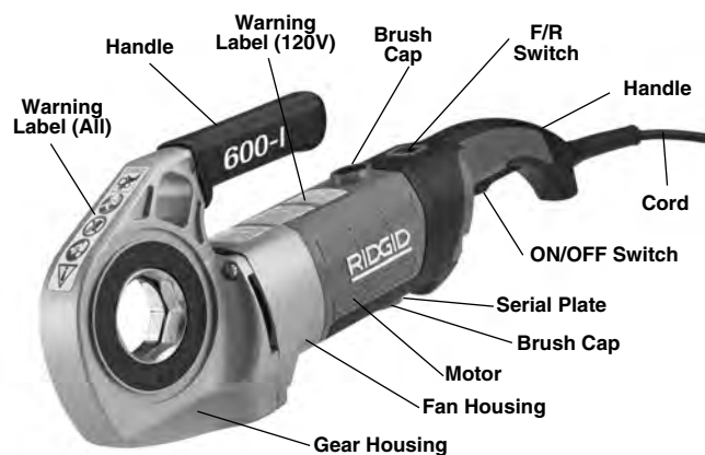
Figure 1 – Model 600-I Power Drive
