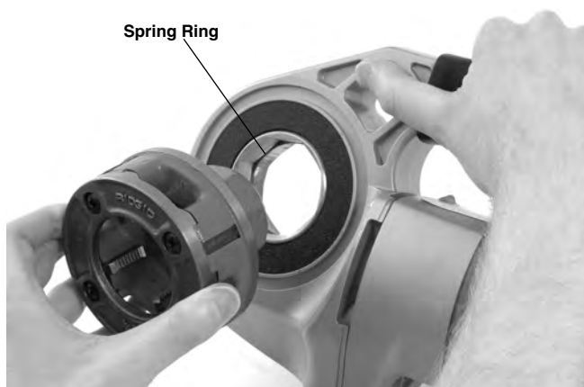
Figure 9 – Installing Die Heads into 600-I Power Drive
