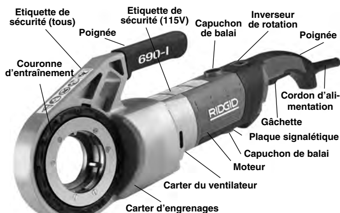
Figure 2 – Fileteuse type 690-I
