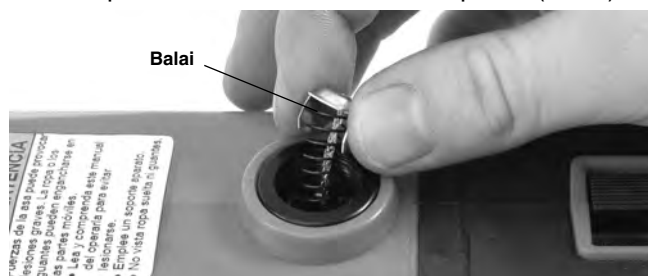
Figure 18 – Installation des balais
