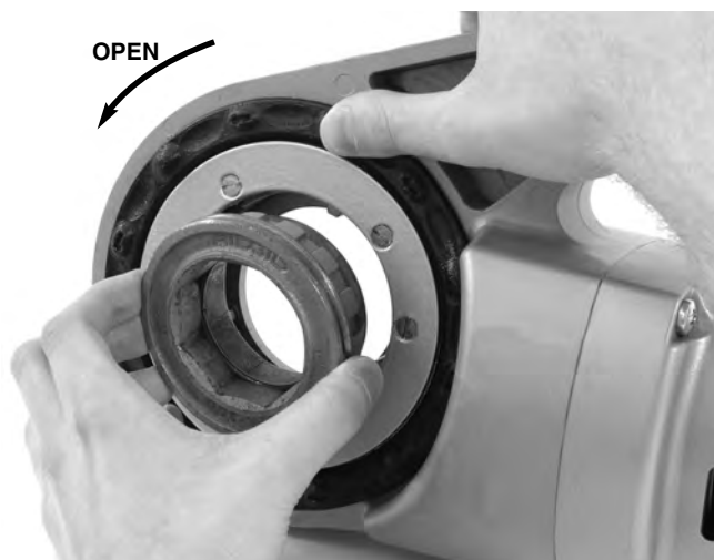
Figure 8 – Installing Adapter Into 690-I
