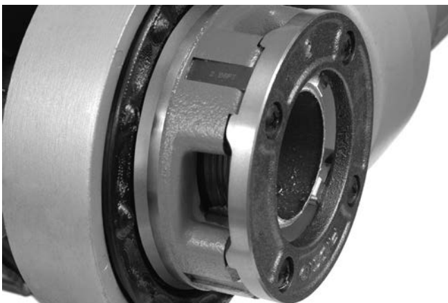
Figure 15 – Pipe Even with Edge of Dies
