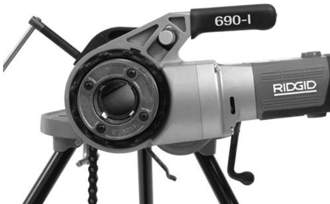
Figure 12 – Proper Orientation of the Power Drive
