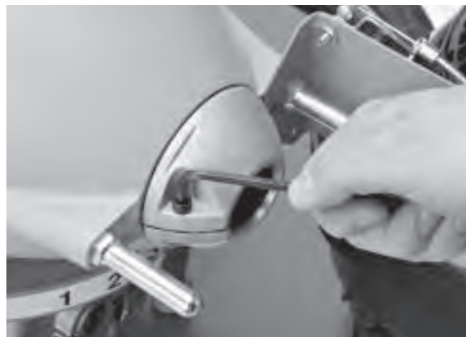
Figure 13 – Removing Clutch End Play
