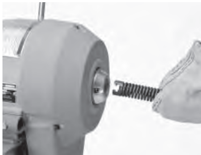
Figure 3 – Inserting Cable Into Front Of Machine
