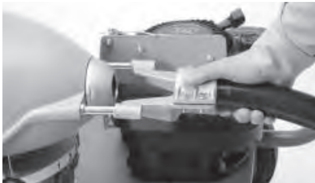
Figure 2 – Raccordement du tuyau arrière
