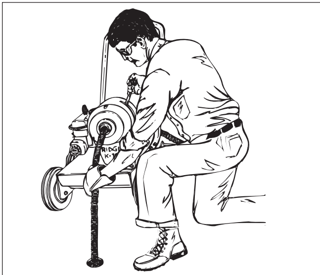
Figure 5 – Operating Drain Cleaning Machine
