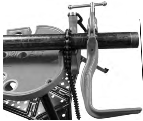
Figure 5 – Support Arm Aligned with End of Pipe
