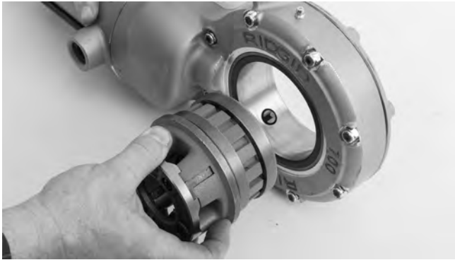
Figure 4 – Installing Die Heads into 700 Power Drive
