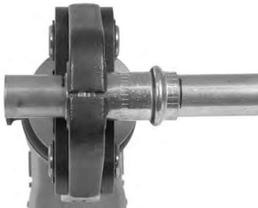
Figure 7 – RP 340 Tool Square To Tubing
