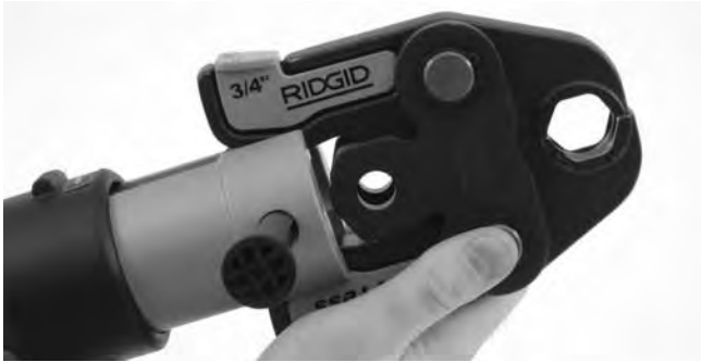
Figure 5 – Slide Attachment Into Tool
