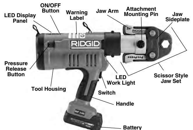
Figure 1 – RP 340 Press Tool and Jaw Set
