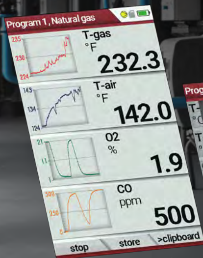
Flue gas Measurement screen with graphics
