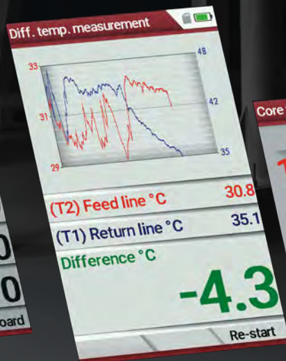
Differential temperature measurement screen
