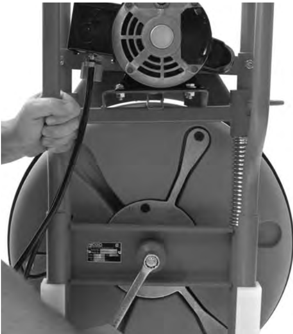
Figure 18 – Removing Drum Bolt
