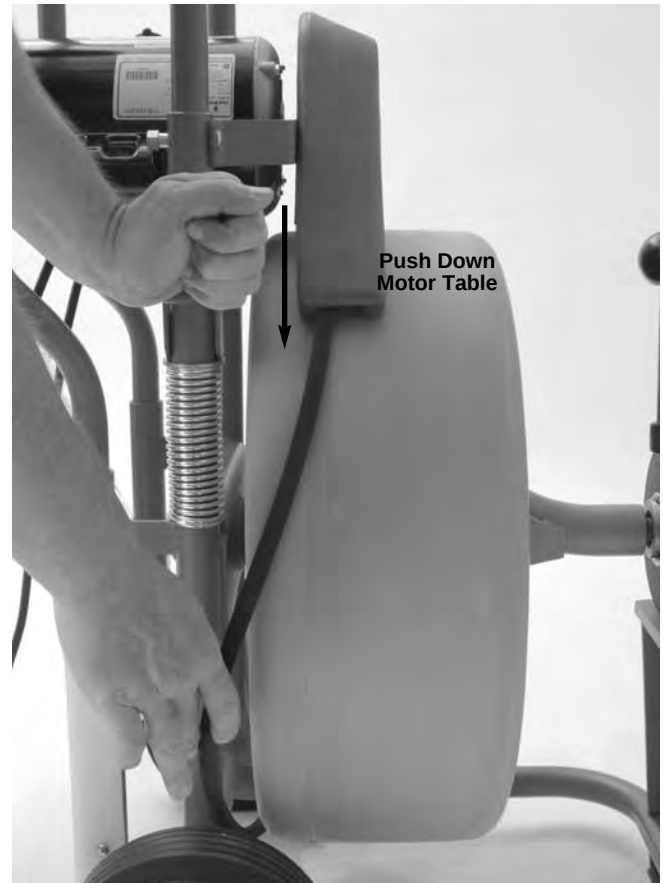
Figure 17 – Releasing Belt Tension
