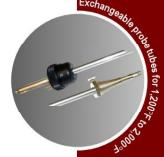
Industrial probe for interchangeable probe tubes with 9' or 16' rugged, braided sheathed sampling line with K-Type t/c and Viton hose for combustion and emission measurements
