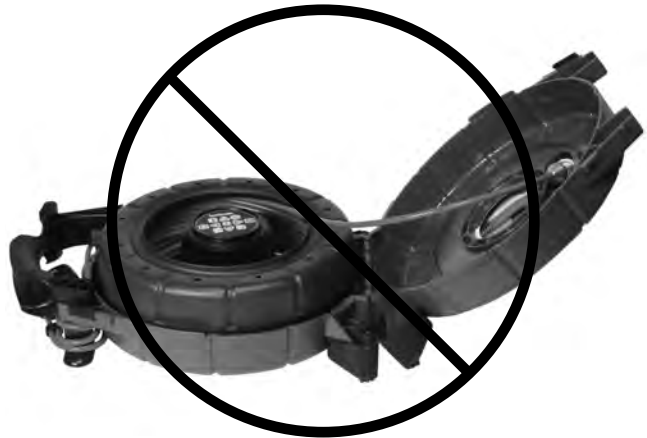
Figure 9 – Do Not Open Case with Camera Outside
