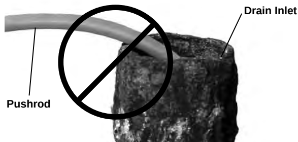
Figure 23 – Avoid Pulling At Sharp Angles
