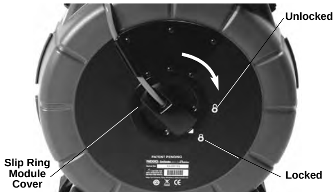
Figure 11 – Locking The Slip Ring Module Cover
