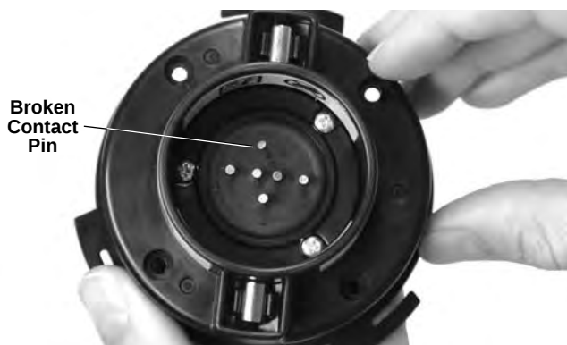
Figure 12 – Broken Contact Pin
