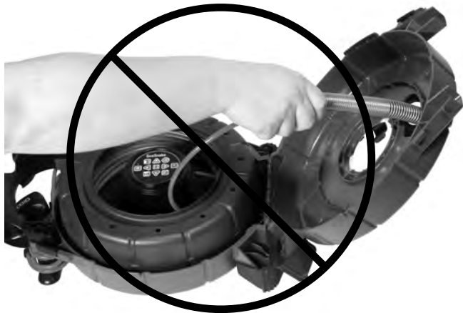
Figure 6 – Do Not Open Case Completely
