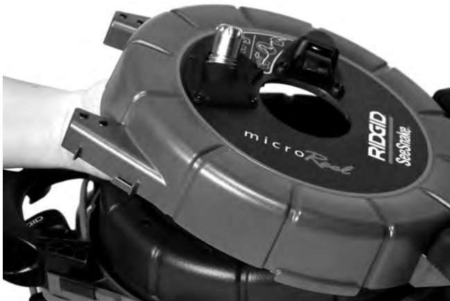
Figure 5 – Open Drum Carefully To Route Cable
