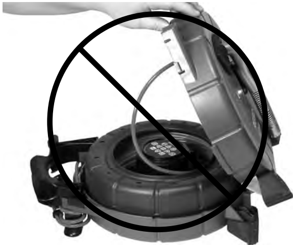
Figure 10 – Do Not Allow Cable to Uncoil Freely
