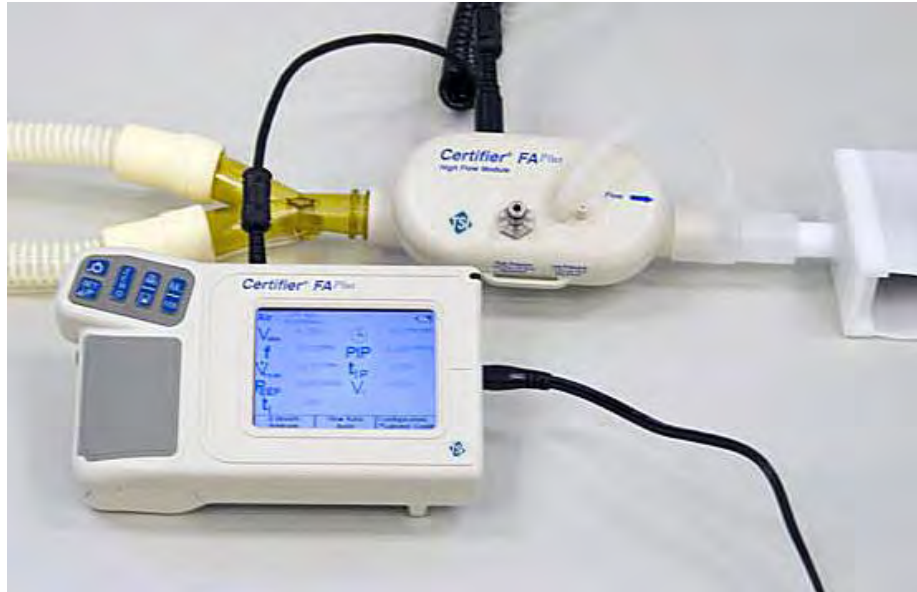
Figure 11. Installing a Flow Module into the Circuit for Measuring Bi-directional Flow
