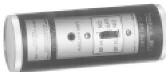
Sound pressure level calibrators are used before or after taking measurements with sound level meters and noise dosimeters.
