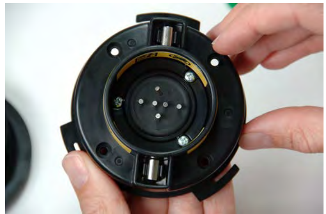
Figure 7 – Broken Contact Pin
