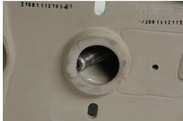
Figure 17 – Camera Head Blocked in Turn
