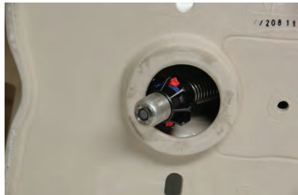
Figure 18 – Camera Head with Ball Guide in Turn
