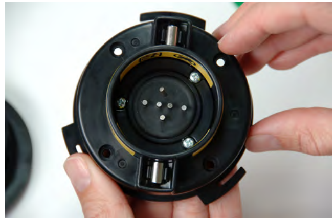
Figure 7 – Broken Contact Pin
