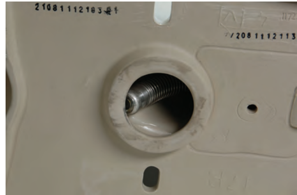
Figure 17 – Camera Head Blocked in Turn
