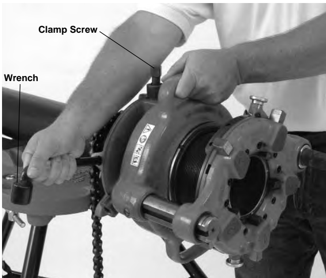
Figure 6 – Tightening Workholder
