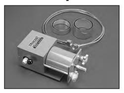
The Frigimat® Dry Ice Maker eliminates the need to buy large quantities of dry ice, producing a solid 16 ounce (454gm) block in one to two minutes. Removing the dry ice block requires just 30 seconds, and the Frigimat® Dry Ice Maker is then ready to make another block of dry ice. Each cylinder of liquid CO2 will make 8 or 9 blocks of dry ice.
