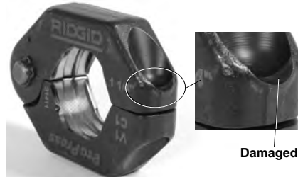
Figure 11 – Damaged Ring Pocket
