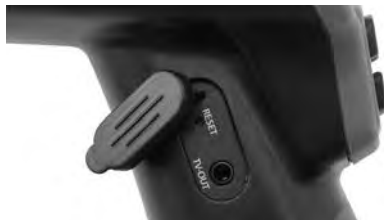
Figure 9 – TV-OUT Jack/Reset Button
