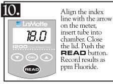
**NOTE:** Zeroing the meter with sample water or an empty chamber will result in an *Er2* message. Meter must be zeroed with a reagent blank.
