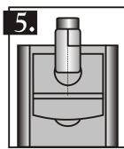
Insert the tube into the chamber, being sure to align the index line with the arrow on the meter. Close the lid. This tube is the sample blank.
