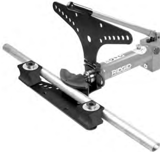
Figure 10 – Loading the Pipe
