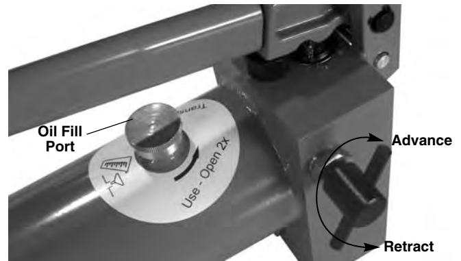
Figure 11 – Release Knob Positions (Advance/Retract)
