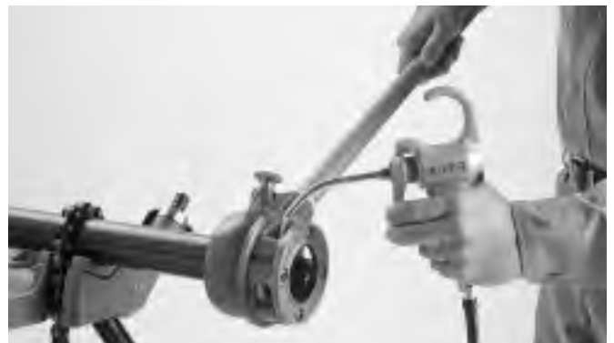
Figure 4 – Applying Thread Cutter Oil
