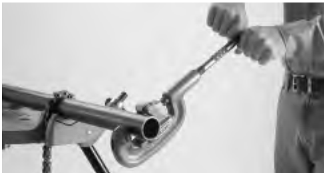
Figure 1 – Cutting End of Pipe
