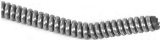
Figure 15 – Bend At Cable End
